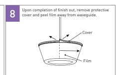
Factory recommends cleaning waveguide assembly with a microfiber cloth or similar non-abrasive cloth. In most cases a damp microfiber cloth will remove dust/debris or fingerprints. For stubborn stains, approved cleaning agents include soap and water, or ammonia based cleaners.
