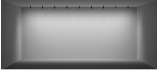
30" SETBACK / 30" ON CENTER SPACING / 10° TILT
