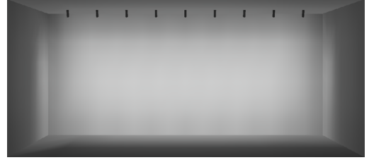
42" SETBACK / 42" ON CENTER SPACING / 20° TILT
