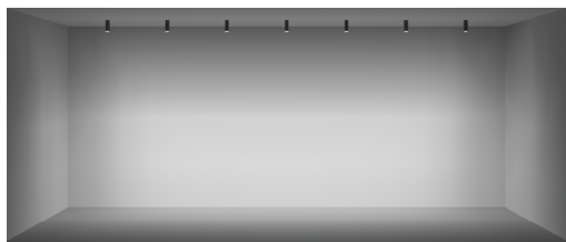
8FT CEILING 36" SETBACK / 48" ON CENTER SPACING
