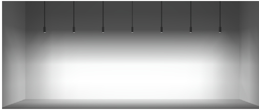
8FT MOUNTING HEIGHT 36" SETBACK / 48" ON CENTER SPACING
