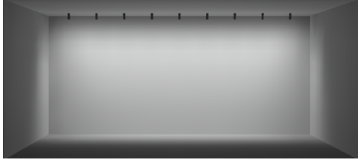
30" SETBACK / 30" ON CENTER SPACING / 10° TILT
