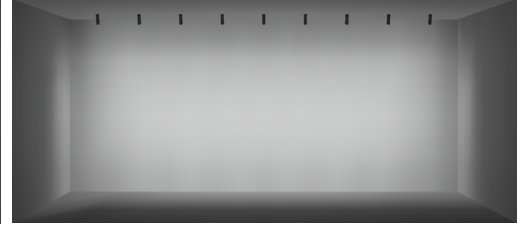
42" SETBACK / 42" ON CENTER SPACING / 20° TILT
