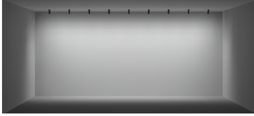
30" SETBACK / 30" ON CENTER SPACING / 10° TILT
