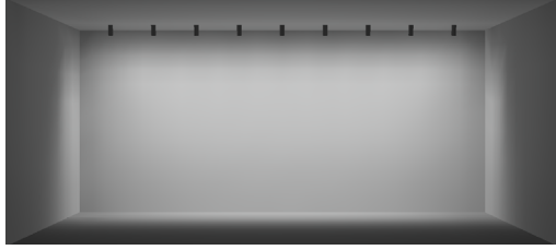
30" SETBACK / 30" ON CENTER SPACING / 10° TILT
