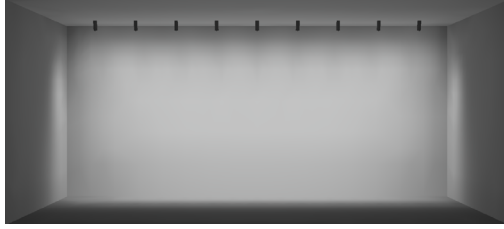
36" SETBACK / 36" ON CENTER SPACING / 15° TILT
