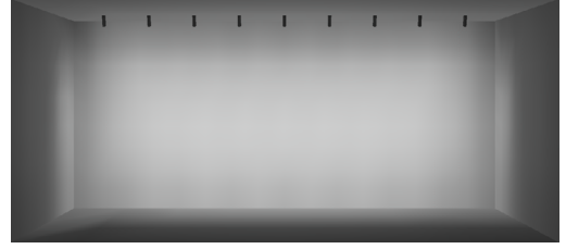
42" SETBACK / 42" ON CENTER SPACING / 20° TILT
