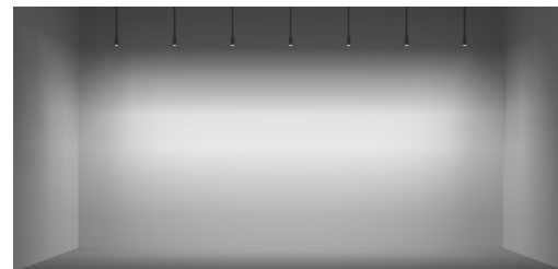
12FT CEILING 36" SETBACK / 48" ON CENTER SPACING
