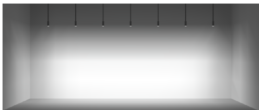
8FT CEILING 36" SETBACK / 48" ON CENTER SPACING
