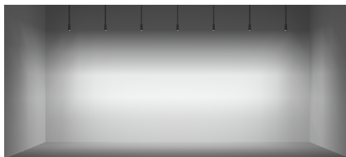
10FT CEILING 36" SETBACK / 48" ON CENTER SPACING
