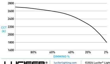
90W11AD 3000K - 1800K Full on 100% Dimmed to 10% Dimmed Dimmed to 50% Dimmed Dimmed Dimmed to 80% to 70% to 20% to 2% CCT (K) 3000 2950 2920 2775 2375 1800 2000 Light Output (Lm) 673 538 471 337 135 67 13 Power (W) 9 11 8 6 2.2 1.1 .2 Efficacy (LPW) 61 61 61 61 61 61 61 90W15AD Full on Dimmed Dimmed Dimmed Dimmed Dimmed Dimmed
